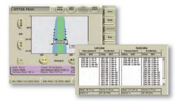
MJSQ-compliant Dual Dirac jitter measurement.
