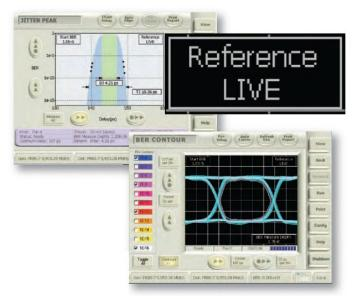
Jitter peak and BER contour measurements made on live data.
