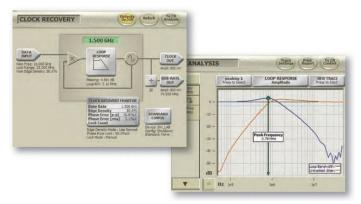
The intuitive user interface provides easy control of all operating parameters. A unique Loop Response view shows the loop characteristics – actually measured, not just the settings value.
