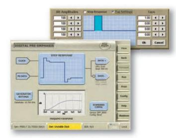
In keeping with the BERTScope philosophy, the graphical user interface presents the control functionality in a logical, easy-to-follow format. A time domain representation of the response shows the effects of tap weight settings. The frequency domain Bode plot shows how the filter will compensate for the channel losses.
