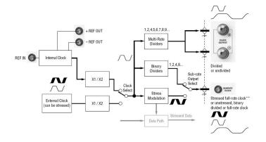
Functional block diagram of the clock path for models with stress capability: BSA125C, BSA175C, BSA286CL.
