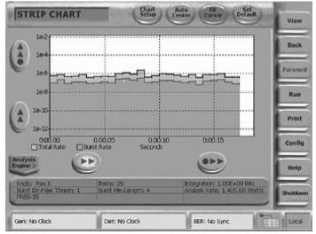
Strip Chart view showing bit and burst error performance over time. This can useful while temperature cycling as part of troubleshooting.
